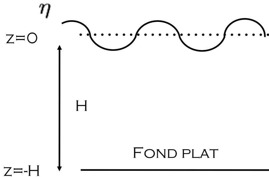
$$\left\{ \begin{array}{l} \partial_t u' + u_0 \partial_x u' + \frac{1}{\rho_0} \partial_x p' = 0 \\ \partial_x u' + \partial_z w' = 0 \\ \partial_z p' = -\rho' g \\ \partial_t \rho' + u_0 \partial_x \rho' + w' \partial_z \bar{\rho} = 0 \end{array} \right. \quad \left\{ \begin{array}{l} \partial_t \eta = w'(0) \\ w'(-H) = 0 \end{array} \right.$$
